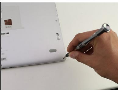
Remove the eight 3 mm screws using the Torx T5 driver by inserting the screwdriver into each screw and rotating counterclockwise.
