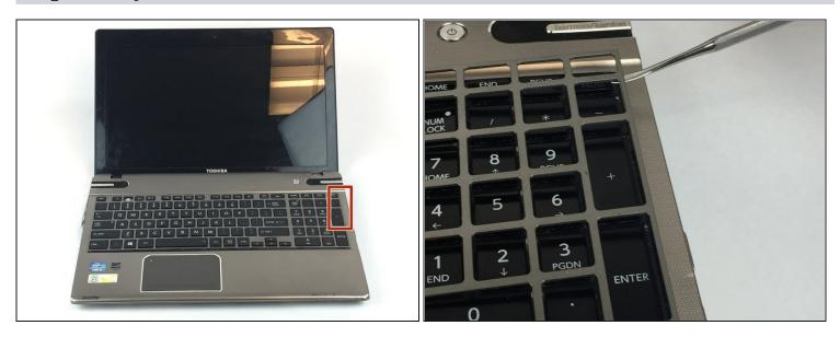
Use a plastic opening tool to pry up the keyboard cover.
