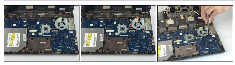
• Remove the three 3mm Phillips #0 screws from the fan.
