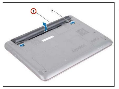
Lift the battery out of the battery bay. After the battery is removed, the left battery latch must be in the locked position.
