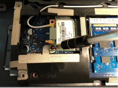
Remove the screw that is securing the wifi card in place
