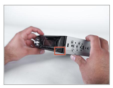
Push the eject button to release the faceplate.
