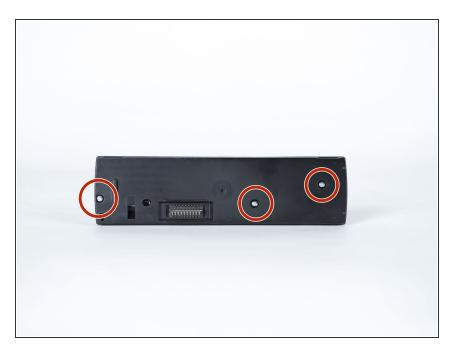
Remove three 3mm Phillips-head screws with a Phillips #1 screwdriver.
