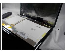
Remove the three M2 5x6 mm screws on each side holding the screen in place, using the Phillips #0 screwdriver.
