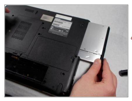
Gently slide the disk drive out to the right until it is removed from the computer.
