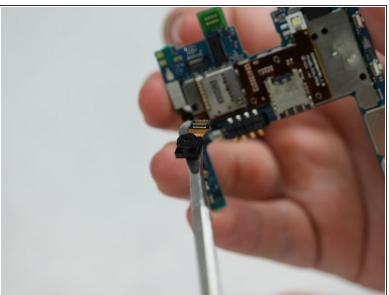
Remove the front camera by its tail with a spudger.
