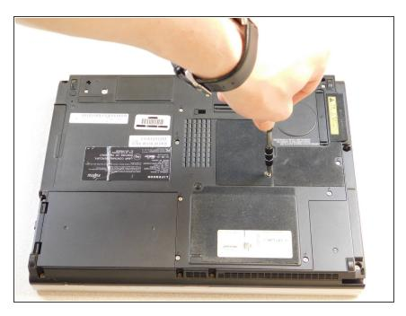
Remove the two Phillips #0 screws from the cover.
