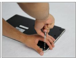
Remove all 14 of the 4 mm screws on the back side of the laptop with a Phillips #1 screwdriver.
