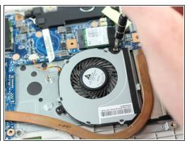
Remove all 4 mm screws with a Phillips #1 screwdriver.
