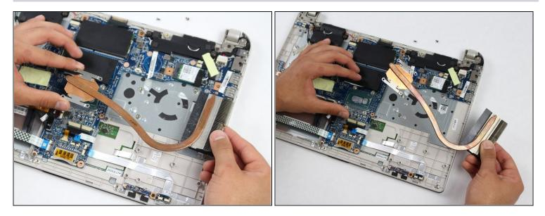
• Carefully remove the heatsink from the rest of the motherboard and casing.
