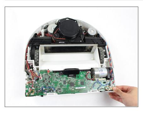
Once you have carefully removed the wire clip; you can fully remove the top cover.
