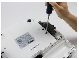
Place the robot on its back and remove the six 11mm screws using a Torx T10 screwdriver.
