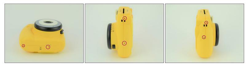
Remove the six 4.5 mm #00 Phillips screws from the bottom, left, and right sides.
