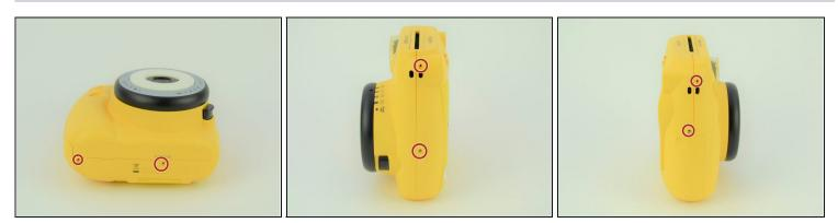
• Remove the six 4.5 mm #00 Phillips screws from the bottom, left, and right sides.
