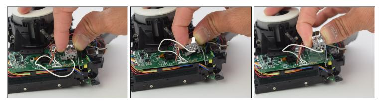
• Remove the flash bulb from the circuit board by shifting it towards the side with the motor and lifting.
