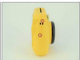
Remove the six 4.5 mm #00 Phillips screws from the bottom, left, and right sides.
