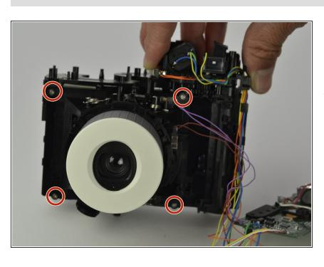
Once the circuit board is off and to the side, remove the four 4.5 mm screws that are around the front lens case using a Phillips #00 screwdriver.
