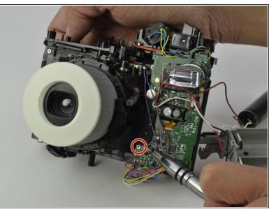
Once the shell is off, remove the two 4.5 mm screws from the circuit board using a Phillips #00 screwdriver.
