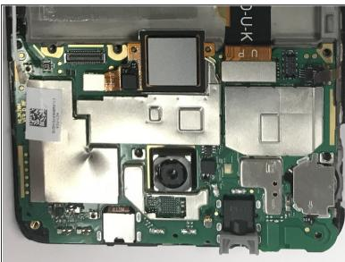
Remove the five 1.5mm Phillips #000 screws from the motherboard.
