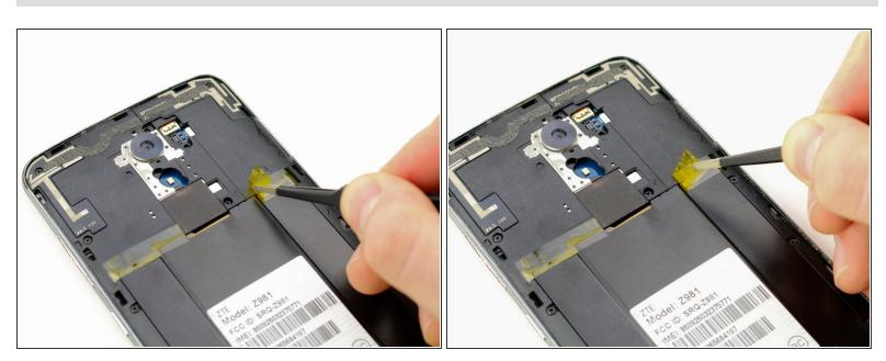
Using the tweezers, peel back the yellow Kapton tape located on the right side of the phone.
