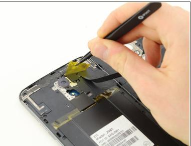
Remove the yellow Kapton tape by using the tweezers to peel it up and away from the device.
