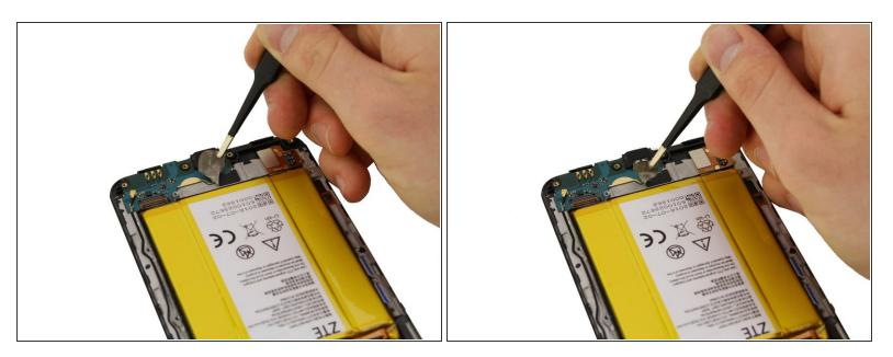
• Use tweezers to peel off the tape at the bottom of the phone.
