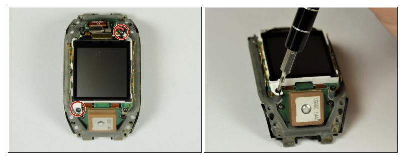
Place a T5 torque screwdriver in the upper right and lower left diagonal 4mm screws that hold the white plastic down and rotate the screwdriver to the left, removing the screws.
