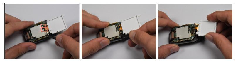
Using tweezers, gently pull the display wiring out of the two connectors that attach the display to the motherboard.
