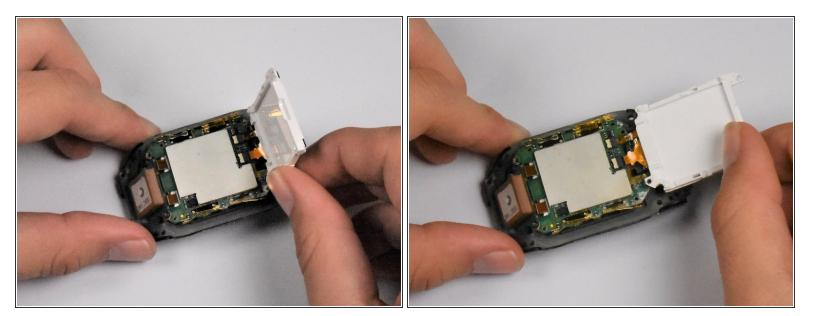
Lift the display from the board from the top side of the watch, revealing the display connectors underneath.
