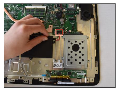
Unplug the battery's connector from the motherboard.
