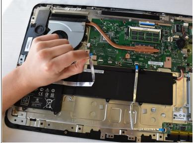
Disconnect the wires by pulling on the tab. Disconnecting these wires will clear the way for removing the battery.
