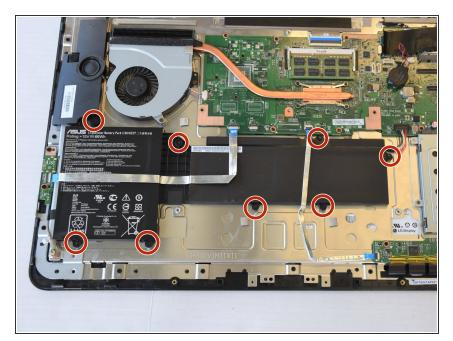
Remove the eight 3.5 mm Phillips screws that secure the battery.
