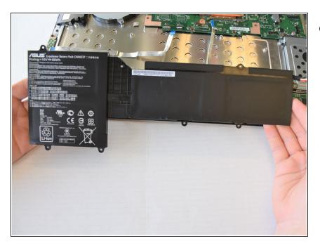
Pull the battery out. Be careful not to break the cables on top.
