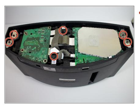
Remove the six 15.5mm PH2 screws securing the grille and rear panel to the device.
