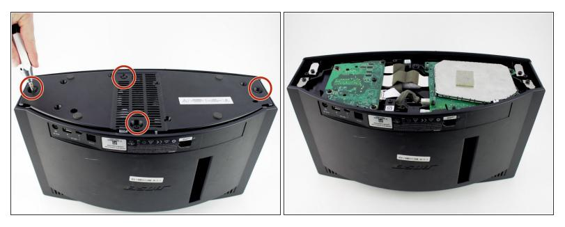
• Remove the four 15.5 mm PH2 screws securing the base plate to the device.
