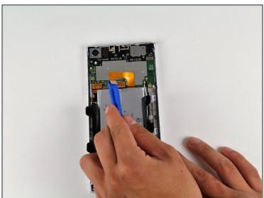
• Use the iFixit Opening Tool to remove the flexible orange strip which connects the battery to the motherboard.
