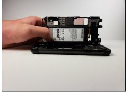
• Use a metal spudger to pull the mid frame and battery off of the motherboard.
