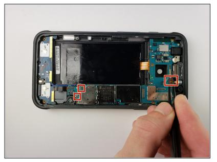
Use tweezers to disconnect the front mic and the two cables that have been marked in the photo.
