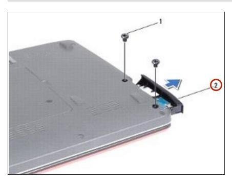
Slide the hard drive assembly out of the hard drive compartment.
