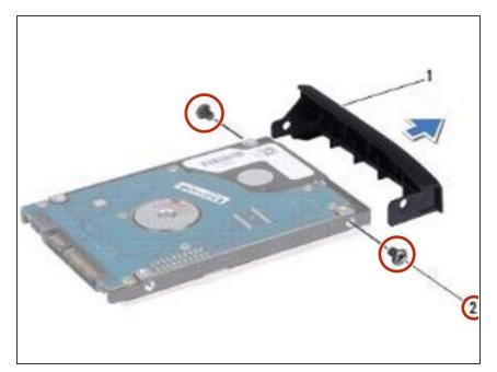
Remove the two screws that secure the hard drive bezel to the hard drive.
