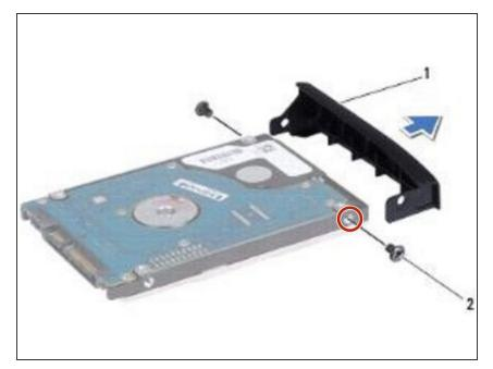
Align the screw holes on the hard drive bezel with the holes on the hard drive.
