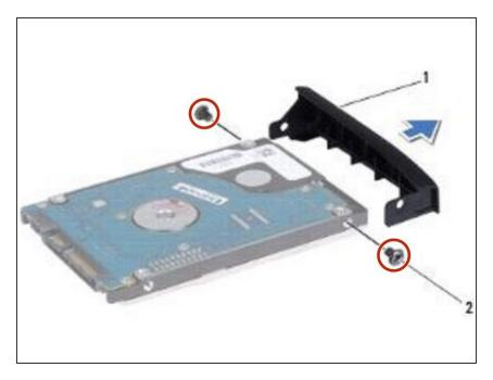
Replace the two screws that secure the hard drive bezel to the hard drive.
