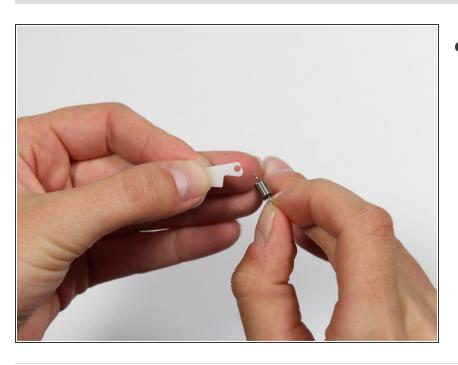
Using two hands, remove the spring from the plastic tabs.
