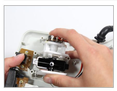
Reach one finger under the guitar to push the whammy bar and its attached components from the case.
