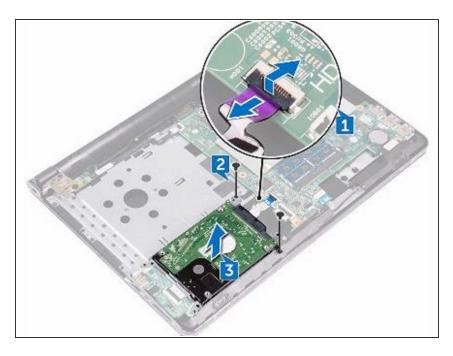
Slide the hard-drive cable into the connector on the system board and press down the latch to secure the cable.
