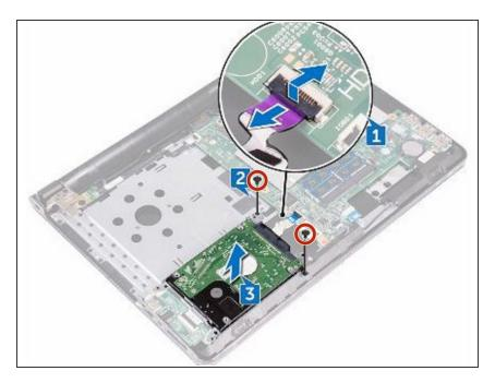
Replace the two screws (M2x3) that secure the hard-drive assembly to the palm-rest assembly.
