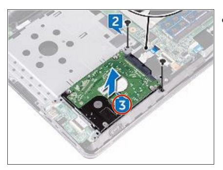
Lift the hard-drive assembly off the hard-drive bracket.
