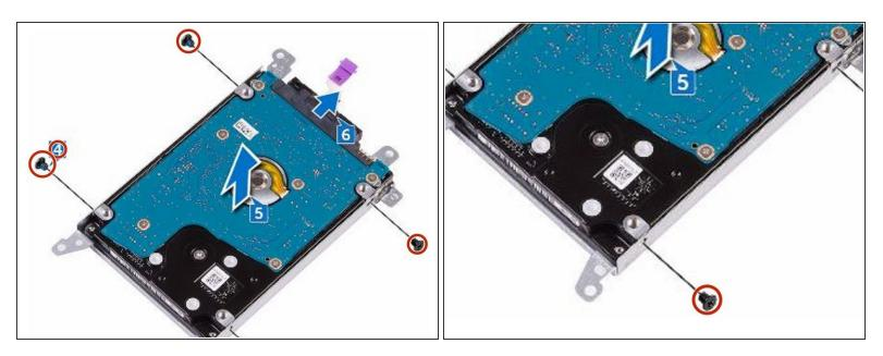
Replace the four screws (M3x3) that secure the hard-drive bracket to the hard-drive assembly.
