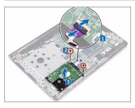
Remove the two screws (M2x3) that secure the hard-drive assembly to the palm-rest assembly.
