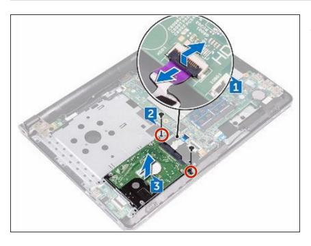
Align the screw holes on the harddrive bracket with the screw holes on the hard-drive assembly.
