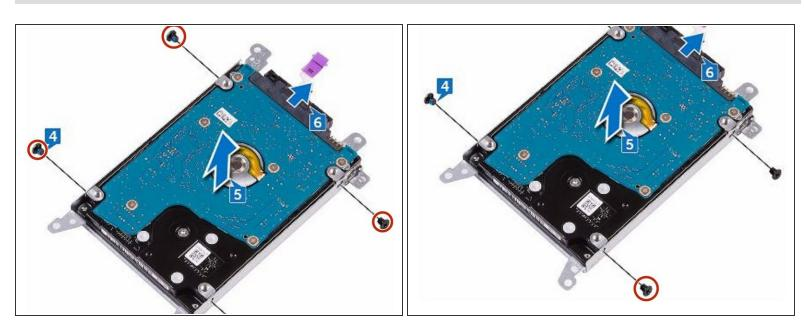
• Remove the four screws (M3x3) that secure the hard-drive bracket to the hard-drive assembly.
