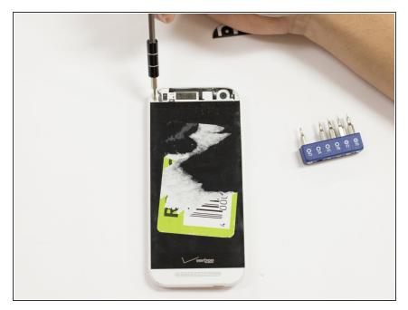
• Take out the small 3 mm screw that is on the top left side using a T5 bit.
