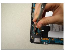
Using the screwdriver, remove the 4 black 3.0 mm Phillips head screws located on the upper and lower motherboard.
