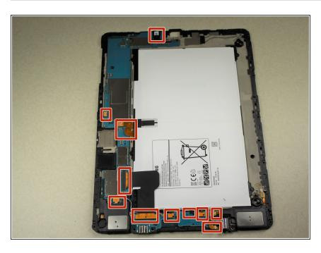
Using the plastic opening tools unlock the 11 connectors that must be undone before the motherboard can be removed.
