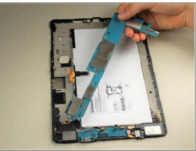
Carefully lift the top portion of the motherboard off of the back panel with your hands.
