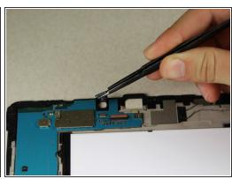
Using the plastic opening tool, continue disconnecting cables on upper motherboard.
