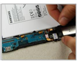
Carefully lift the orange flap using the black spudger. Then disconnect the cable from the motherboard.
