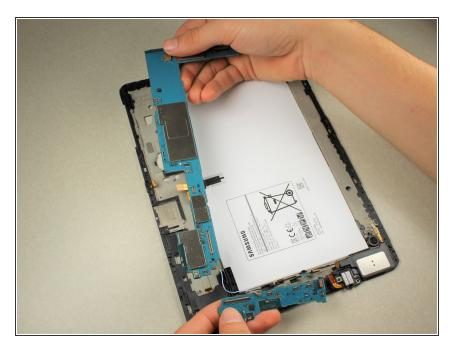
Remove both pieces of the motherboard carefully from the back panel. To reassemble your device, follow these instructions in reverse order.
