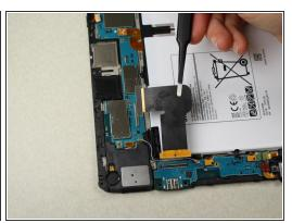
• Using the tweezers, gently pull the cable off of the motherboard.
