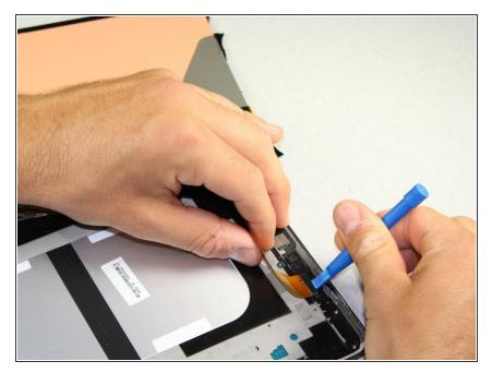
Use the plastic opening tool to get under the connector piece. This will allow you to remove the front panel assembly from the rest of the device.
