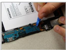
Continue removing cables on the lower motherboard.
