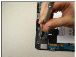
• Using the screwdriver, remove the 4 black 3.0 mm Phillips head screws located on the upper and lower motherboard.
