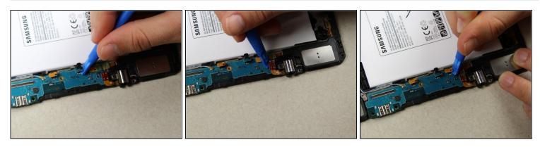
• Continue removing cables on the lower motherboard.
