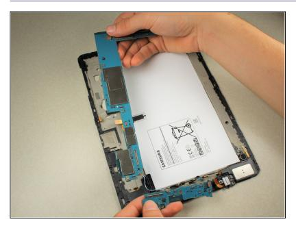
Remove both pieces of the motherboard carefully from the back panel.
