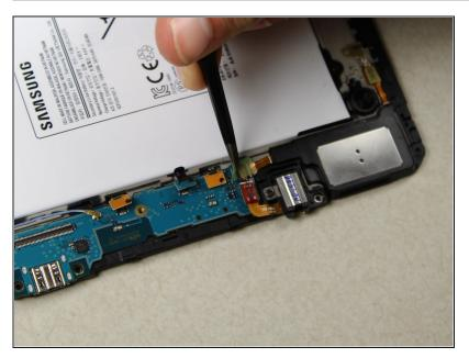
Using tweezers, remove the green plastic film to reach the last cable.
