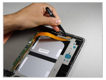
Using the tweezers, gently peel up on the silver tape covering the connector.
