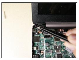
• Lift the tarp material straight up off the external output using tweezers. It is simply taped on.
