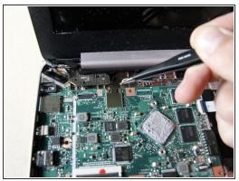
Pop these two connections off by using tweezers to lift straight up.
