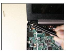
• Lift the tarp material straight up off the external output using <u>tweezers</u>. It is simply taped on.
