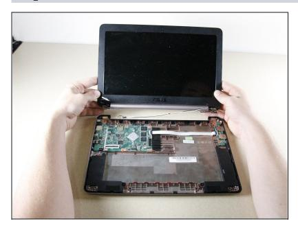
• Lift the screen up to fully remove.
