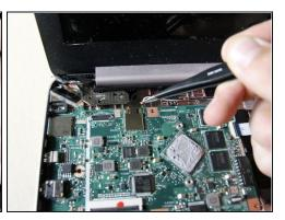
• Pop these two connections off by using tweezers to lift straight up.
