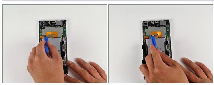
• Use the iFixit Opening Tool to remove the flexible orange strip which connects the battery to the motherboard.
