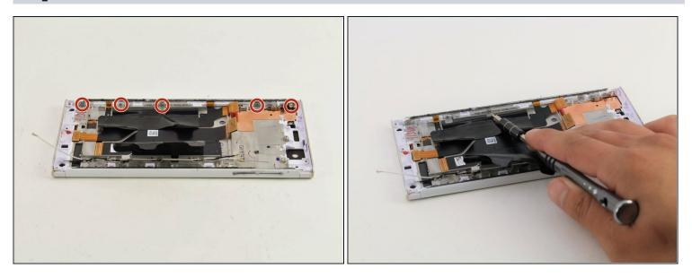
• Remove the five 4mm T5 screws connecting the SD card side panel to the device.
