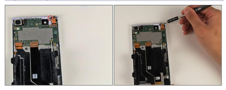
• Remove the 4mm T5 screw connecting the headphone jack to the panel.
