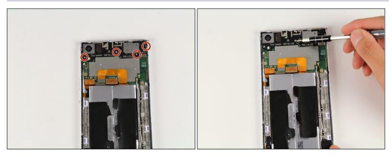
• Remove the four 4mm T5 screws on the top of the black panel securing the antenna module to the device.
