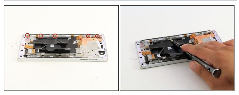
• Remove the five 4mm T5 screws connecting the side panel to the power button flex cable.
