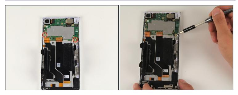
• Remove the two 4mm T5 screws connecting the motherboard to the device.
