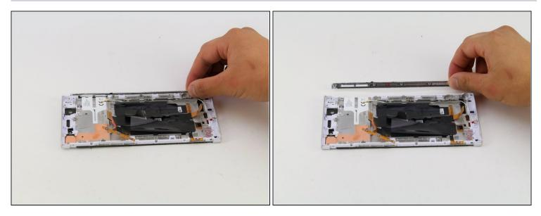
• Remove the SD card side panel from the device by grabbing the SD card side panel with your hands and sliding the SD card side panel away from the device.
