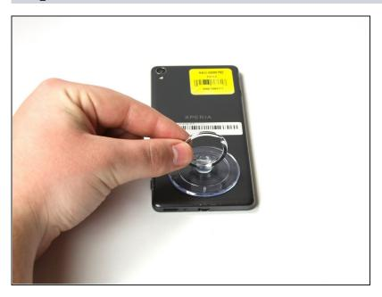
Stick the small suction cup on the bottom half of the back surface of the phone.
