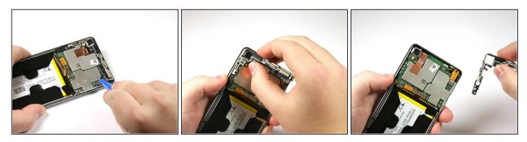
• Pry up the black camera case with the plastic opening tool and then remove the case.
