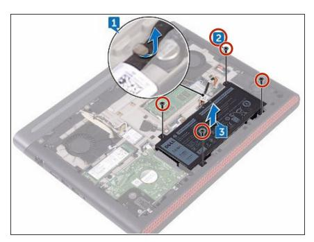
Remove the four screws (M2x4 T8) that secure the battery to the computer base.
