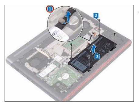
• Route the battery cable through the routing guide on the computer base.
