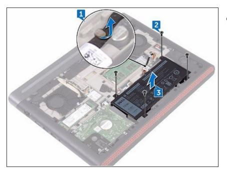
Align the screw holes on the NEW battery with the screw holes on the computer base.
