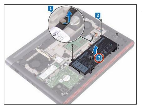
• Lift the battery off the computer base.
