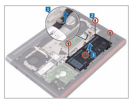
Replace the four screws (M2x4 T8) that secure the battery to the computer base.
