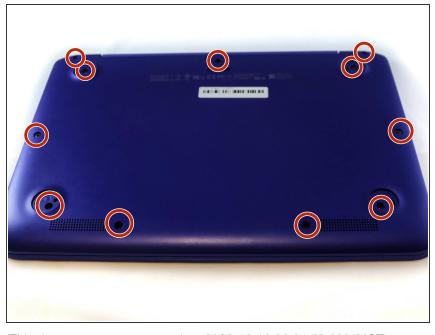
Using the Phillips #1 screwdriver, remove all eleven of the 5mm screws.
