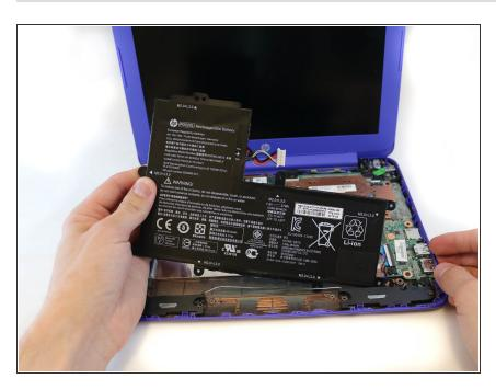
Gently lift and pull the battery out of the device. To reassemble your device, follow these instructions in reverse order.
