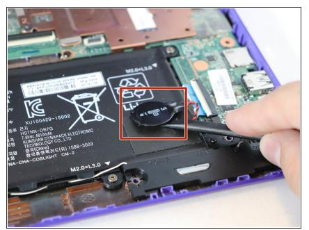
With the black nylon spudger lift the small circular battery off of the main battery.
