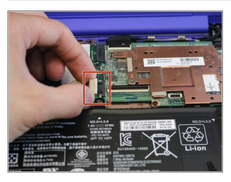
Lift the battery cable free from the motherboard with your fingers.
