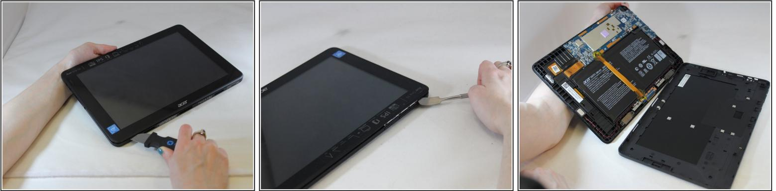
**i** While handling the device, make sure to avoid pushing the power button. Device must remain powered off.
