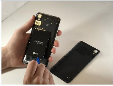
Insert the plastic opening tool into the indent below the battery, and pry up to lift and remove the battery.
