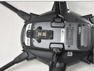
Lift all drone arms up so you can access the landing gear easily.
