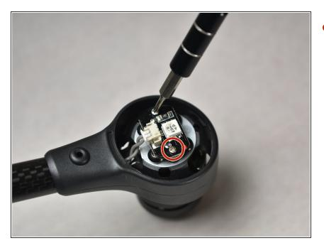
Unscrew two 4.9mm screws on the board using a Phillips #000 screwdriver.
