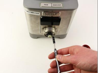
• Using a Phillips #1 screwdriver to remove the three 3/8" screws holding the selector bezel in place.
