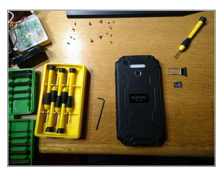
Unscrew 8 side screws (flat 2.4mm or dedicated torx), then 4 rear screws (hex 1.5mm).
