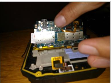
Remove the stuck SIM card.
