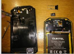
Withdrawal of back of phone and unplugging of LED connector.
