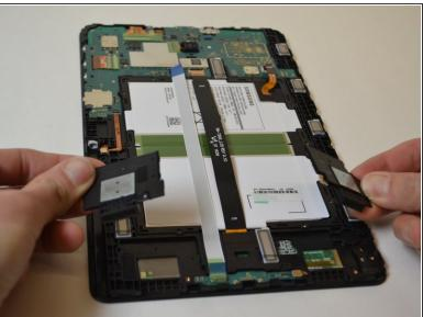
Use a plastic opening tool to pry the speakers out of the tablet
