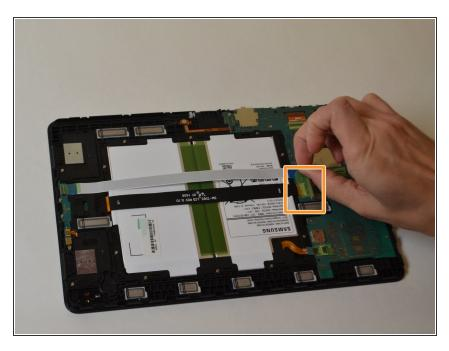
Use a spudger to flip up the retaining flap on the ribbon cable <u>ZIF</u> socket.
