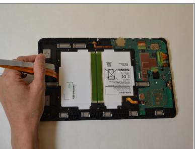
Remove the ribbon cable from the socket.
