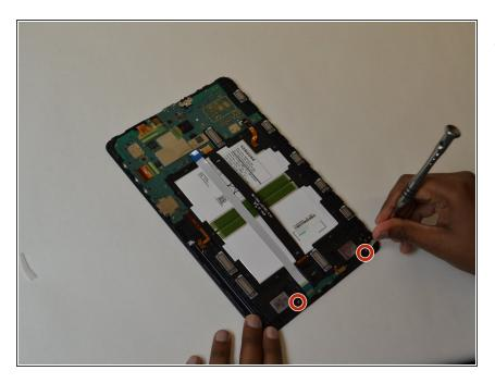
Remove the two 4mm Phillips #000 screws from the speakers.
