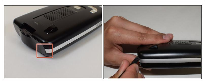
Inser the flat end of a spudger into one of the two notches and pry off the case.
