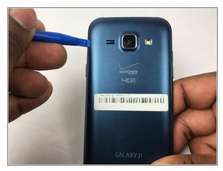
Using a plastic opening tool, gently pry the plastic backing off the body of the phone.
