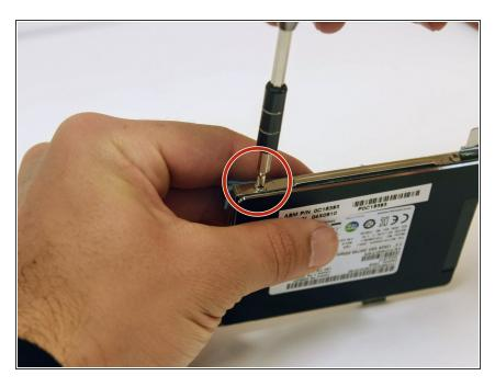
Remove the four M3 x 3 mm, flathead, nylon-coated screws on the side of the hard drive assembly using the Phillips #0 screwdriver.
