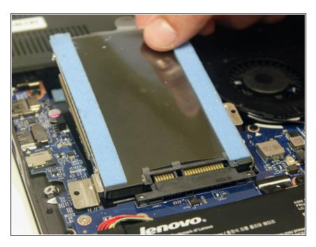
Pull the hard drive assembly out with backside up.
