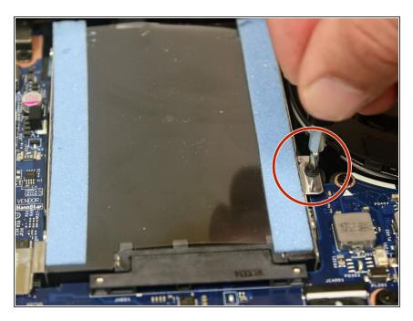
Remove the two M2 x 3 mm, waferhead, nylon-coated screws that hold down the hard drive assembly using the Phillips #0 screwdriver.
