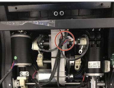
Now we need to disconnect the wire harness from the mechanism. Do this by simply unplugging the marked cables
