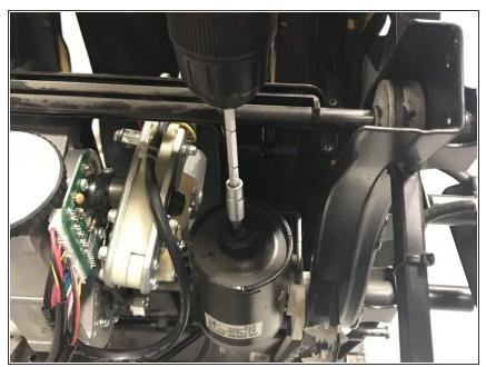
Next attach a flat head bit to a cordless drill and insert it into the the top of the Up and Down motor. this will allow you to drive the mechanism out the top of the track.
