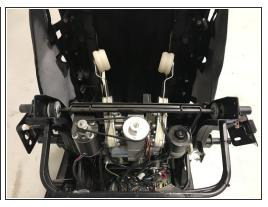
Remove all 4 screws on top bar
