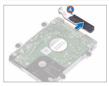
• Disconnect the interposer from the hard-drive assembly.
