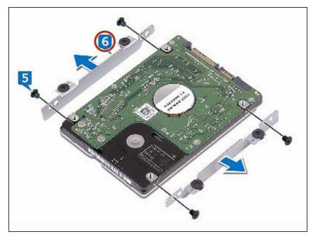
• Remove the hard-drive bracket off the hard drive.
