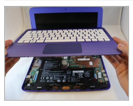
After detaching the two large ribbon cables, carefully lean the keyboard against the screen.
