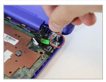
Using the Phillips #1 screwdriver, remove the 4 mm screw.
