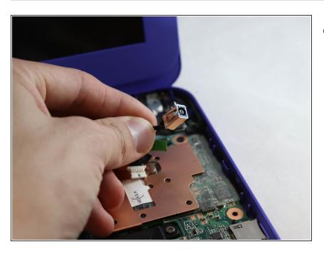
Lift and remove the charging port from the device.
