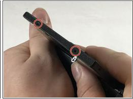
Remove the six 2mm Phillips #000 around the edge of the screen.
