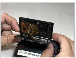
Using the plastic opening tool, pry back the backplate from the front of the screen.
