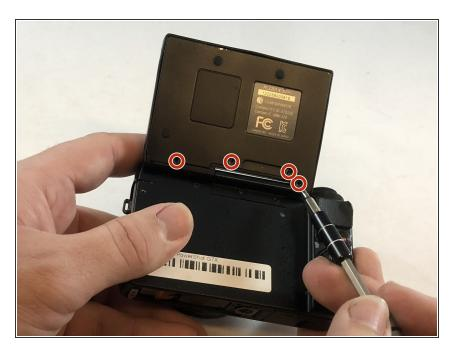
Remove the four 2mm Phillips screws from the back of the screen.
